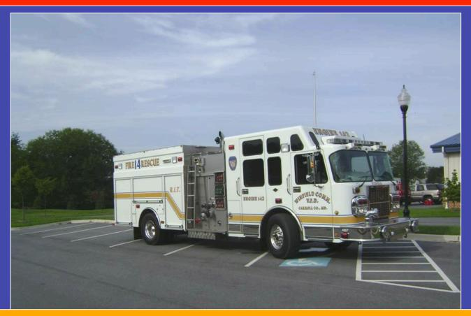
Winfield Community VFD's Engine 142 – a 2007, 4-Guys pumper with a Hale 1,500 gpm single-stage, QMax pump and a 4-inch high-flow discharge.
