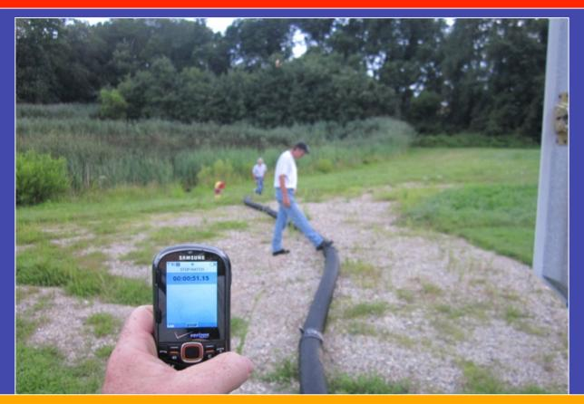
At the 51-second mark, water had traveled 50 feet through the suction hose and the test was well on its way to a better result than Flow Test #1.
