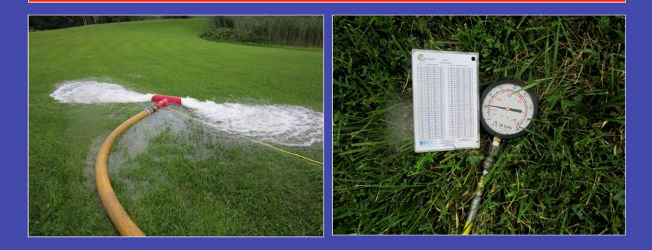
The Hose Monster recorded a pitot pressure of 22 psi which converts to 791 gpm.
