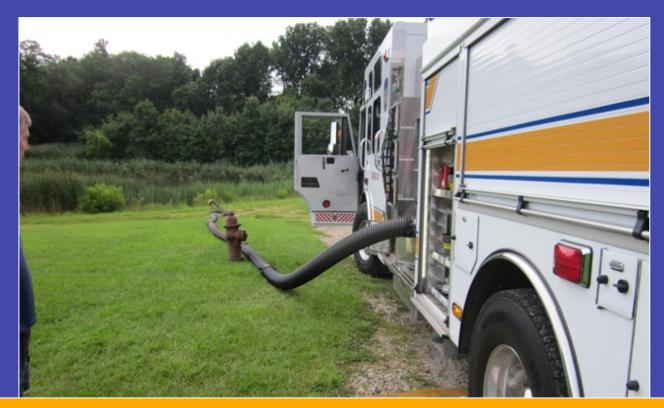
The total lift was less than 10 feet – however, an absolute measurement was not obtained. Disregard the fire hydrant in the foreground – it is an old, out of service hydrant.
