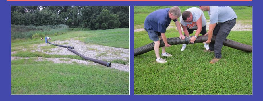
100-feet of 6-inch hard suction hose was connected to the driver side 6-inch suction intake on Engine 142. The other end of the suction hose was connected to a 6-inch dry fire hydrant at a local pond.
