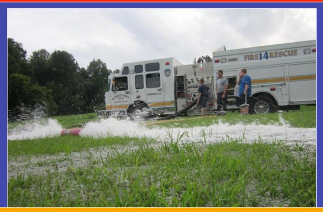
The Hose Monster pitot recorded a pressure of 36 psi which converts to 1,012 gpm – which is pretty good given the 100 feet of suction hose!
