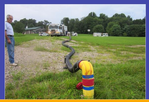
There were many air bubbles seen in the suction hose during the test. The dry hydrant was checked and a significant air leak was found at the swivel. The air leak could not be fixed so the operation was switched to a floating strainer.
