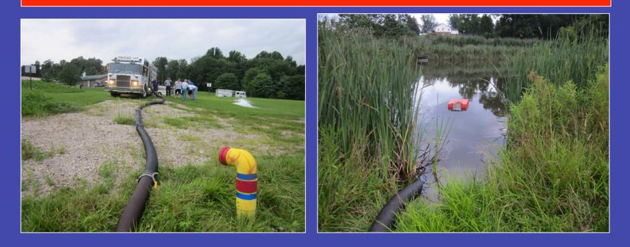
The 100 feet of suction hose was disconnected from the dry hydrant and reconnected to a 6-inch floating strainer. Flow Test #2 was ready to begin.
