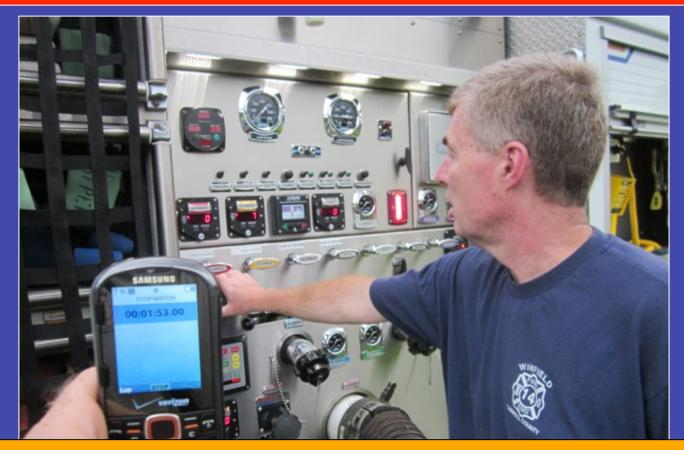
Time was stopped at 1:53 minutes when water reached the pump and discharge pressure registered on the pump's master discharge gauge.
