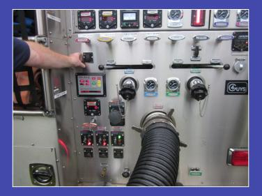
Time was started when the driver pushed the air primer's control switch. Time was stopped at 2:40 minutes when the pump was primed and discharge pressure was noted on the master discharge gauge.
