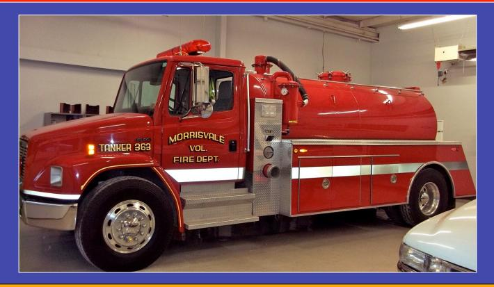
The test vehicle was a 1994 Firovac vacuum tanker. The tanker carries 2,000 gallons of water and has three, 6-inch dumps – one on each side and one in the rear.
