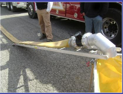
An in-line gauge was installed in hopes of capturing a pressure reading, but that was not successful because of the large opening and no resultant backpressure which to measure. A folding ladder was used to support the 5-inch hose and reduce kinking.
