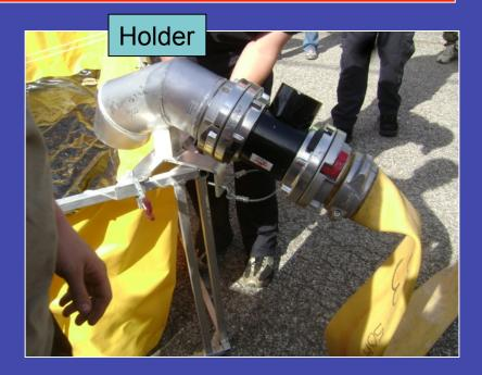
A 2,500-gallon dump tank was set up as a "catch basin" for the water that was going to be offloaded. A 100-ft length of 5-inch LDH was outfitted with a supply line holder device so that the hose would be held firmly in place at the dump tank during the test.
