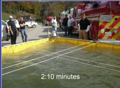
Water flowed through the 5-inch LDH and out into the dump tank with little effort. At the 2:10-minute mark, all of the water was exhausted and air began exiting the end of the 5-inch hose – thus the test was over and time was stopped.
