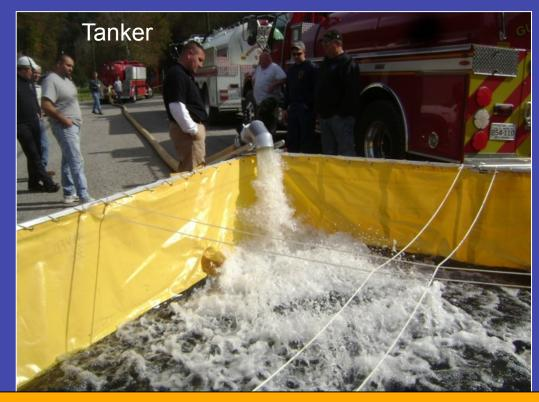
On the timer's signal, the tanker operator engaged the vacuum pump and started the offloading process. Water was offloaded into the 5-inch LDH using the tanker's rear, 6-inch dump.
