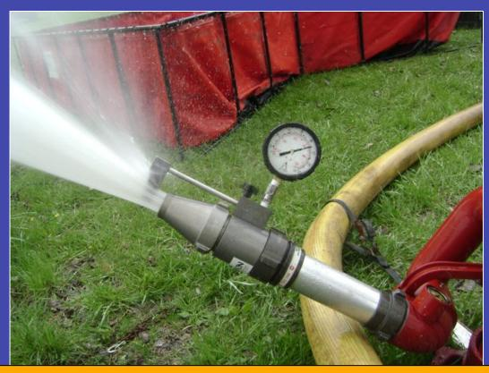
With Turbo Draft feeding the pumper, the portable monitor produced an effective fire stream.
