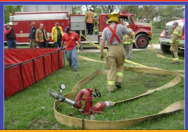
A portable monitor was once again used – but this time it received its water from the pumper.
