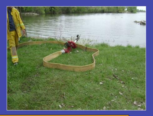
This test attempted to measure the Turbo Draft's flow potential when being fed by 3-inch hose. The objective was to measure the flow at the portable monitor.
