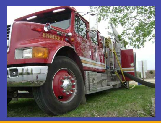
Lincolnville Engine 1 – a 1,500 gpm pumper w/1,000 gallon tank was used to support each flow test.
