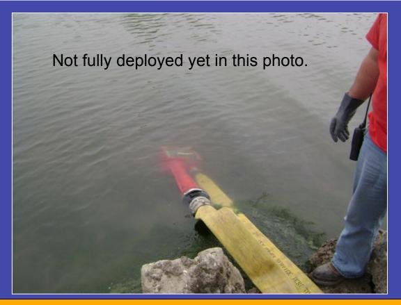
The Turbo Draft was submersed in about 2-feet of water and rested on the lake's rocky bottom.
