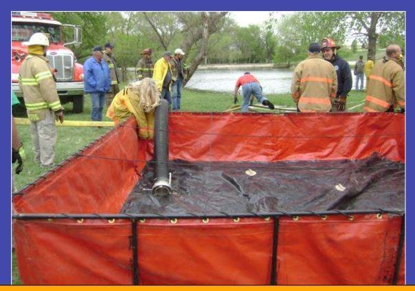
While less scientific than Test #1, the goal with Test #2 was to see how fast the test set-up could fill a 3,000 gallon portable dump tank
