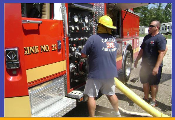
Calera Engine 22 – a 1,500 gpm pumper w/1,000-gallon tank – was used as the source pumper for Flow Test #2.
