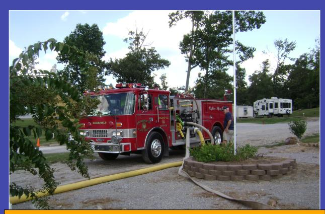
Brierfield Engine 203 – a 1,500 gpm pumper w/500 gallon tank was used as the source pumper in the first flow test.
