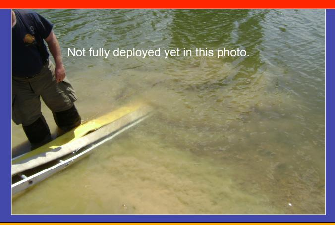
The Turbo Draft was submersed in about 2-feet of water and rested on a roof ladder because of the lake's silted bottom.
