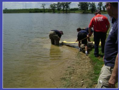
The Turbo Draft was placed on a roof ladder to aid in deployment. The device was fed by 100-feet of 3-inch hose and the device returned water to the pumper through 100-feet of 5-inch hose.
