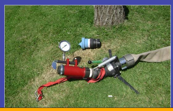
Flow measurement for both tests used a fixed pitot attached to a portable master stream device. The pitot was equipped with a 1-1/2-inch tip and the master stream device was fed by 3-inch hose from the source pumper.
