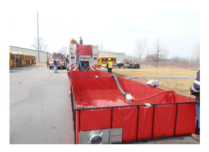
Side dump tankers could top off all four dump tanks in a single pass.
