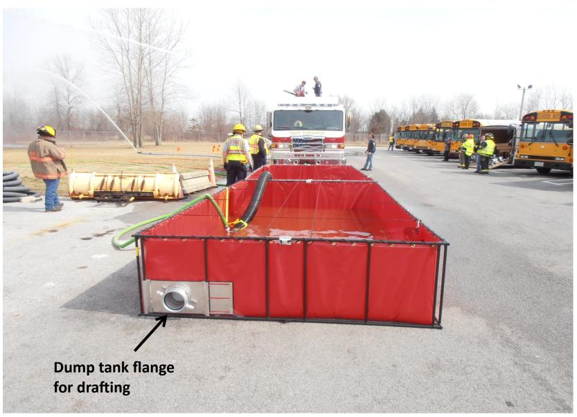
Five (5) vacuum tankers delivered 863 GPM. It appeared that this setup of four 2,000 gal. dump tanks could handle fire flows of 1,000 GPM —the key would be a steady even flow of tankers. With so many tankers with side dumps operated from the driver's seat there was very little need for people to operate dump valves in the dangerous tanker travel lane.
