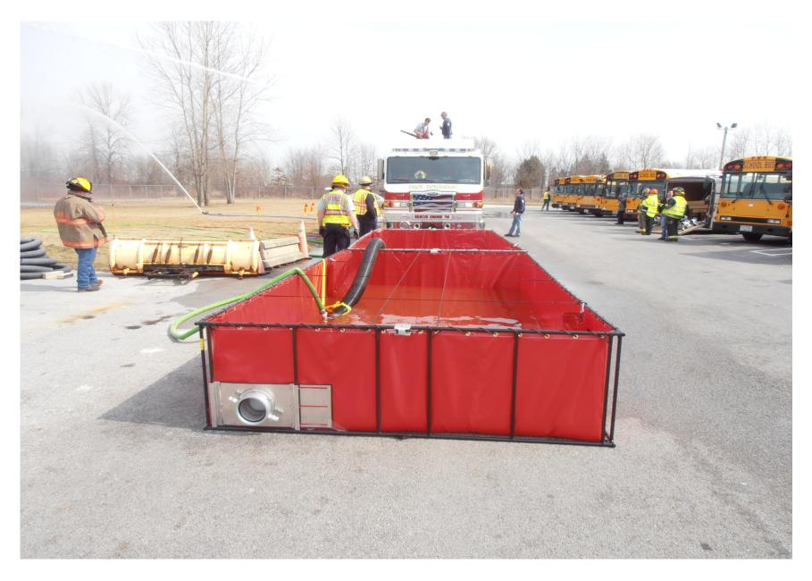
...two rectangular dump tanks behind the pumper —all in a single traffic lane.
