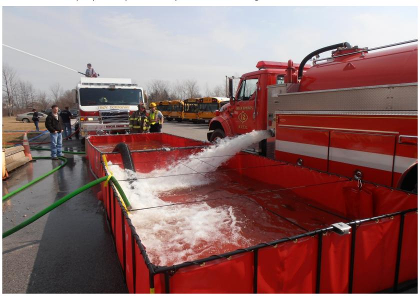
As this side dumping vacuum tanker works its way down the line of dump tanks it could safely dump into the drafting tank. The rectangular dump tanks are 8 ft. wide X 14 ft. long. The suction low level strainer was in the corner of the dump tank. Tankers dump in the other end of the dump tank about 10 ft. from the strainer. The turbulence of the tanker dumping didn't bother the low level strainer. In fact the tankers dumped in the drafting tanks first!
