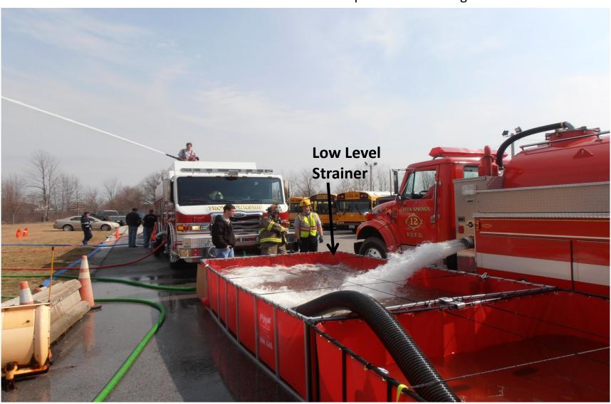
The passenger (officer) side suction drafted from the two dump tanks to the rear of the pumper. The driver side suction drafted from the front two dump tanks.
