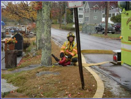
A TFT Crossfire portable monitor was fed by a 100-ft section of 4-inch hose. The nozzle was a 2-inch smooth bore. The master stream device was anchored to the tree for safety.
