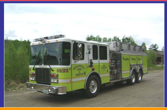
25-Engine-3 is a 2008, Ahrens Fox 1,750 gpm engine/tanker with a 3,000 gallon tank. It has a 500 hp Cummins motor and a single-stage Waterous pump. The unit carries 1,200 ft of 4-inch hose, has a 10-inch rear dump/fill, and is equipped with a 3,500 gallon dump tank.
