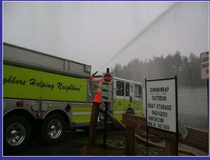
Pitot reading of 88 psi. Flow of 1,114 gpm
