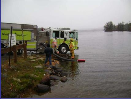
The engine/tanker was nosed down the boat ramp as far as possible in order to minimize lift. Dual, 6-inch suction hoses were used, each 15-ft in length – and one connected to each side of the pump.
