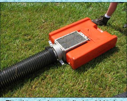
Floating strainer as it should look compared to one which has been plugged by vegetation - which actually collapsed the strainer, making it useless
