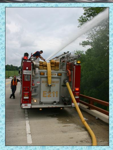
The flow from the pumper's prepiped deck gun was near 900 gpm. A hand held pitot gauge was used to verify the flow through the 2-inch tip.
