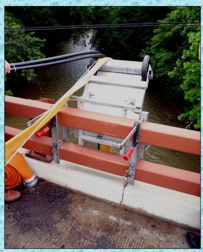
A problem that arose early on into the test was the winch cable, hydraulic hoses, and 4-inch supply hose getting tangled.
