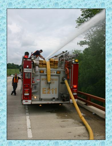
The Mini clearly demonstrated its ability to pump water and overcome head pressure issues. The use of the 4-inch hose made it easy for the pump to deliver the 900 gpm at 16.5 psi PDP.
