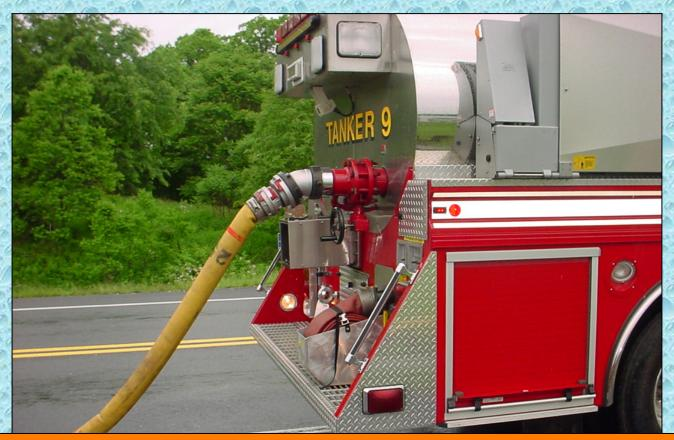
The 3,500 gallon tanker was filled in 3:57 minutes - a rate of 875 gpm.
