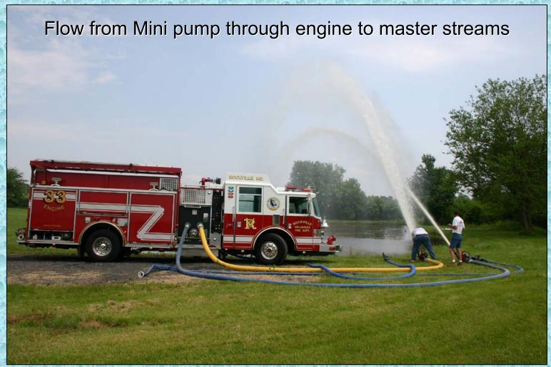
Engine discharges through 5" and 3" lines to master stream devices
