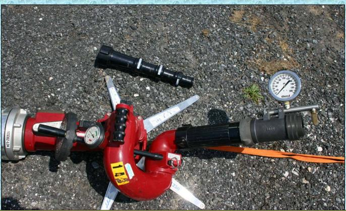
TFT Crossfire with smoothbore and pitot gauge to measure flow
