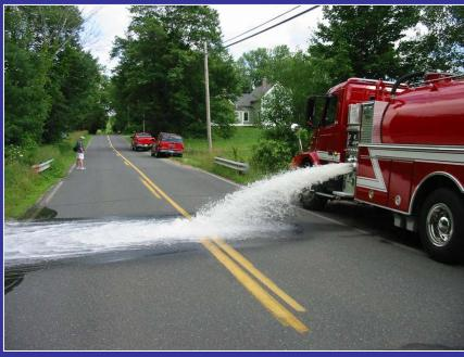
Vacuum tankers have become more popular in recent years, primarily for their ability to refill without the need for additional personnel or equipment. The Granby FD leadership tested the vacuum tanker shown above and was impressed with its overall ability to move water with limited manpower.
