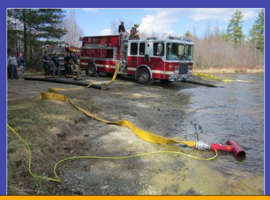
20-feet of 6-inch hard suction hose connected to the driver side 6-inch suction intake. Suction strainer was a Kochek floating strainer. Hose Monster flow diffuser is seen in foreground..
