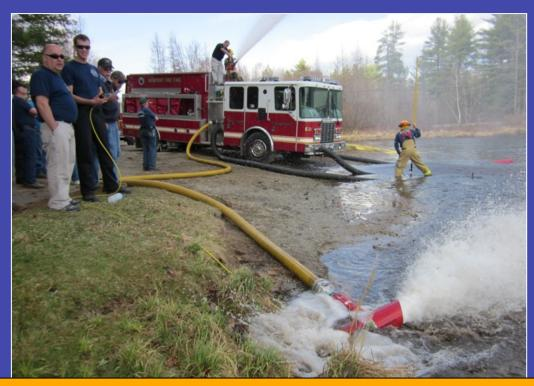
No change to the driver side and officer side set-up. Twenty feet of 6-inch hard suction hose was added to the 6-inch front intake. A 6-inch box strainer was used.
