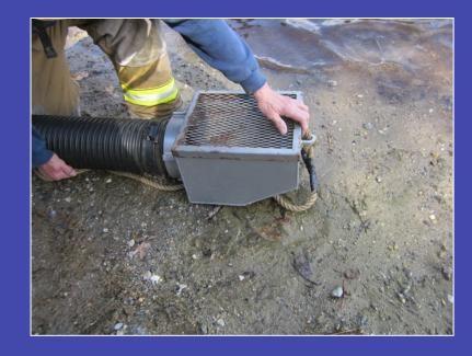
No change to driver side suction set-up. Added 30-ft of 6-inch hard suction hose on officer side 6-inch suction intake. A 6-inch box strainer was used.
