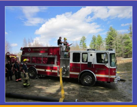
Newport Fire & EMS's 88 Engine 2 — a 2002 Ferrara engine/tanker with a Hale 1,500 gpm single-stage QMax pump and a 4-inch high-flow discharge.
