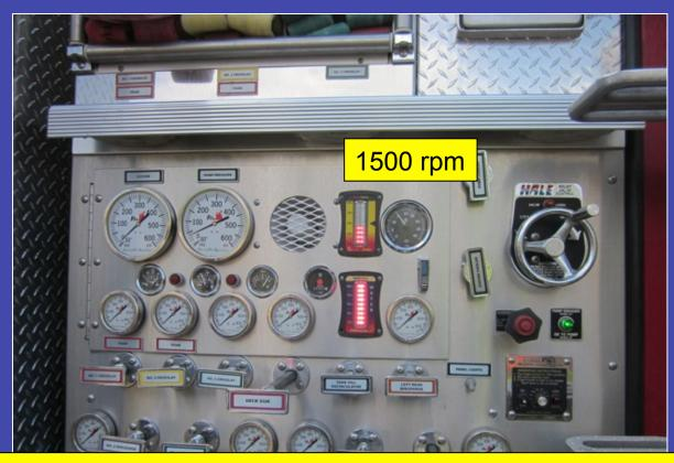
For each test, the throttle was increased until a reading of 1500 rpm was achieved on the tachometer. At that point, flow measurements were recorded.
