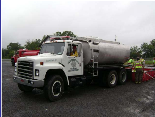
Cartersville T1 – 2,500 gallons
