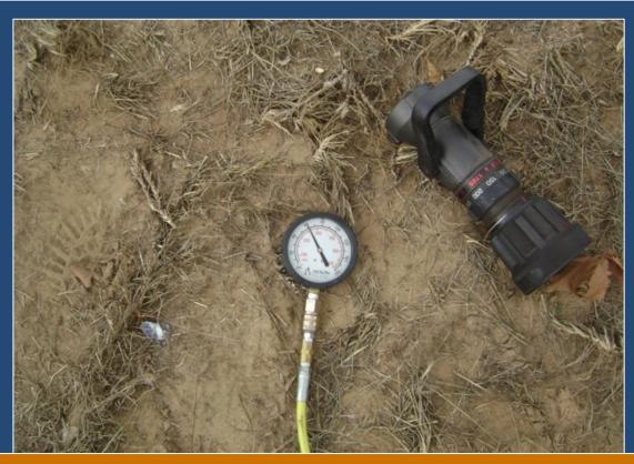
With a pitot pressure reading of 62 psi on the 1-3/4-inch tip, a flow of 701 gpm was achieved. Engine 902's master discharge gauge read 235 psi and the individual discharge gauge read 160 psi.
