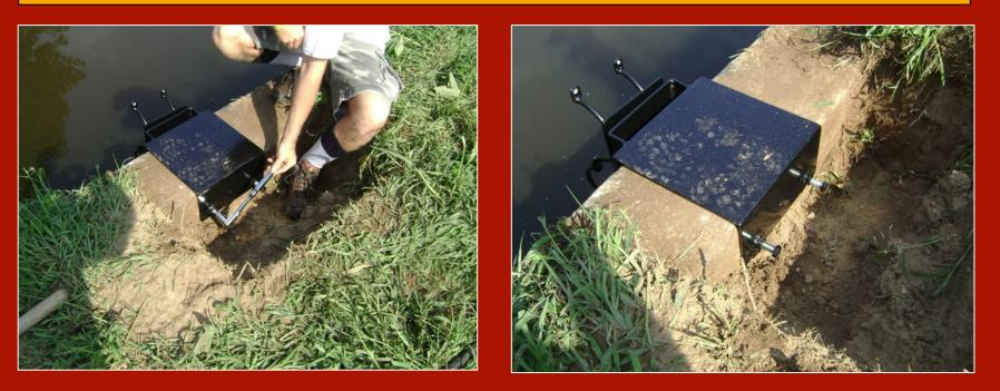
Made of ¼-inch, hot rolled steel and powder coated for protection, this heavy-duty bracket insures a rigid mounting system without the need for drilling holes. The two bolts shown are "tension" bolts that are "snugged" up against the concrete abutment to prevent any side to side motion.
