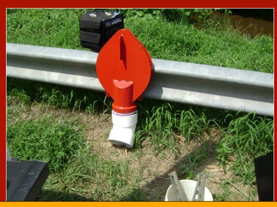
A Kochek 6-inch teardrop style strainer was used as the suction strainer on this system. This strainer works well in shallow, moving water – thus a good choice for this project.
