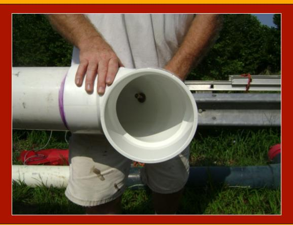
The nut end of the eye bolt protrudes very little into the elbow and thus does not obstruct the flow.
