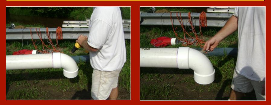
Another important fabrication step was installing the retrieval system for the deployable pipe. A simple, stainless steel eye bolt was used in the lower elbow of the pipe. Later, a length of rope will be attached to that eye bolt in order to control the strainer end of the pipe during deployment and retrieval.
